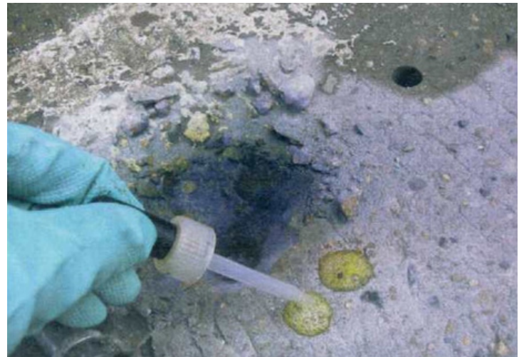
BELOW (left): Dilapidated seawall, with exposed and rusting rebar ; BELOW (right): Corrosion testing being completed on seawall concrete.
