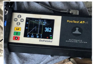
The test was performed according to the ASTM 4541 testing guidelines
