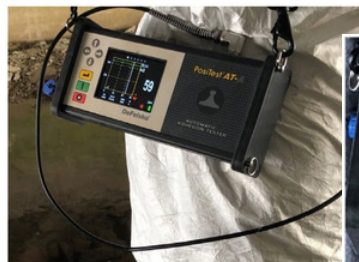
The test was performed according to the ASTM 4541 testing guidelines
