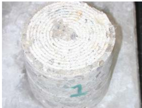
Figure 6: Abrasion surface grooving of sample 1
