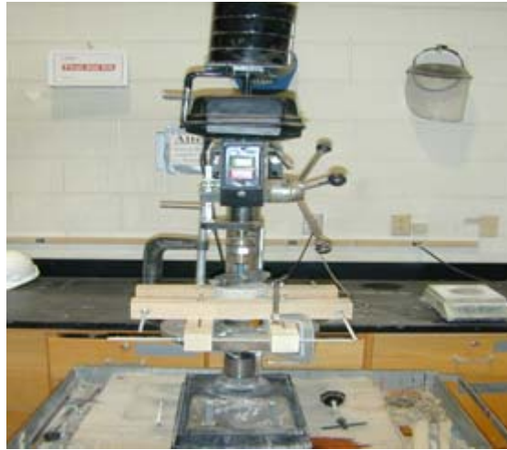
Figure 5: Sample secure and normal to drill press shaft
