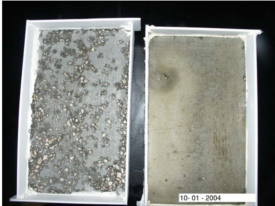
Figure 3: Untreated (left) and treated (right) samples after exposure to 50 freeze-thaw cycles.
